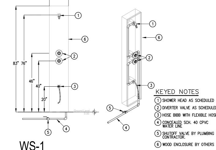
1) SHOWER HEAD AS SCHEDULED 2) DIVERTER VALVE AS SCHEDULED 3) HOSE BIBB WITH FLEXIBLE HOSE 5 SHUTOFF VALVE BY PLUMBING CONTRACTOR.
