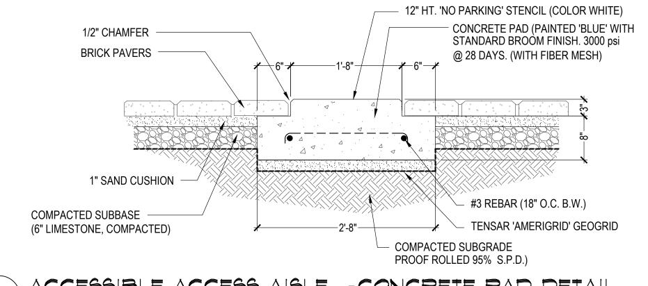
ACCESSIBLE ACCESS AISLE -CONCRETE PAD DETAIL
