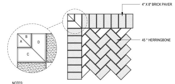
1. DIMENSIONS SHOWN ARE FOR A 90° CORNER. ADJUST DIMENSIONS ACCORDINGLY FOR OTHER ANGLED CORNERS. 2. ALL MITER CUTS TO BE EVEN AND CONSISTENT.
