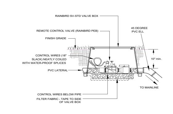
ALL VALVE BOXES SHALL HAVE FILTER FABRIC AND 4" OF GRAVEL AT BASE
