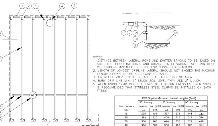
XFS SUB-SURFACE DRIPLINE END FEED LAYOUT INST. N.T.S.
