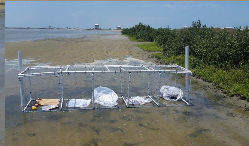
Each containment unit has 5 separate compartments. Four of those compartments are used to hold one lantern burned at a certain percentage. The last compartment housed an apple, a peach, a piece of cardboard, and a paper bag.
