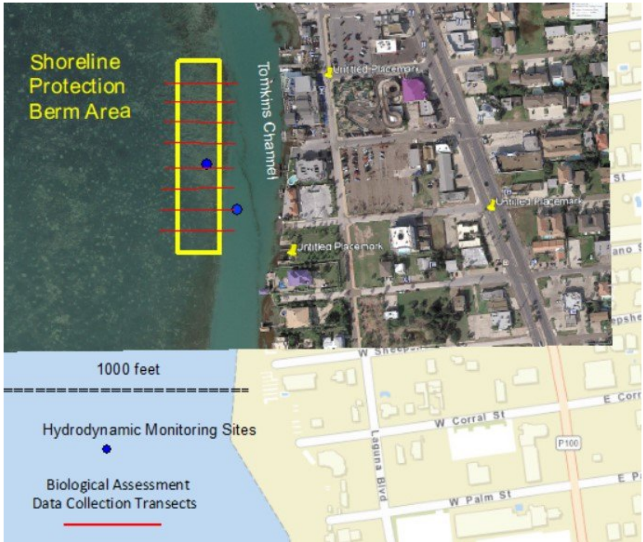
Figure 2. Map showing location of proposed shoreline protection berm area, hydrodynamic monitoring sites, and biological assessment data collection transects
