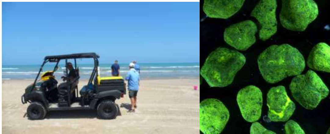
Figure 2. a. Collection of sand samples for tracer analysis on South Padre Island Beach; b. Innovative 'dual signature' (fluorescent and magnetic) natural sand particles used to track sand movement.
