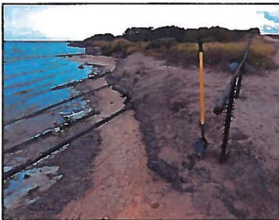
Conducting sediment/soil sampling of the Baffin Bay shoreline in order to evaluate erosion patterns.
