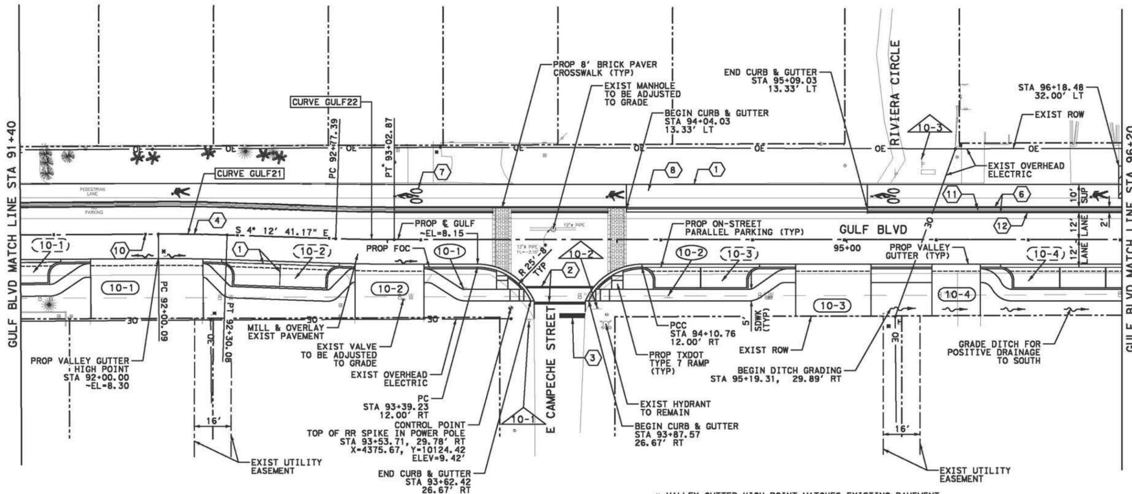
\* VALLEY GUTTER HIGH POINT MATCHES EXISTING PAVEMENT ELEVATION. CONTRACTOR TO FOLLOW EXISTING PAVEMENT SLOPE FROM PROP GUTTER HIGH POINT TO BAHAMA ST. CONTRACTOR TO MILL APPROXIMATELY 37 SY OF ADDITIONAL PAVEMENT (3" MAX) BETWEEN PROP GUTTER HIGH POINT AND CAMPECHE ST TO MAINTAIN POSITIVE DRAINAGE.
