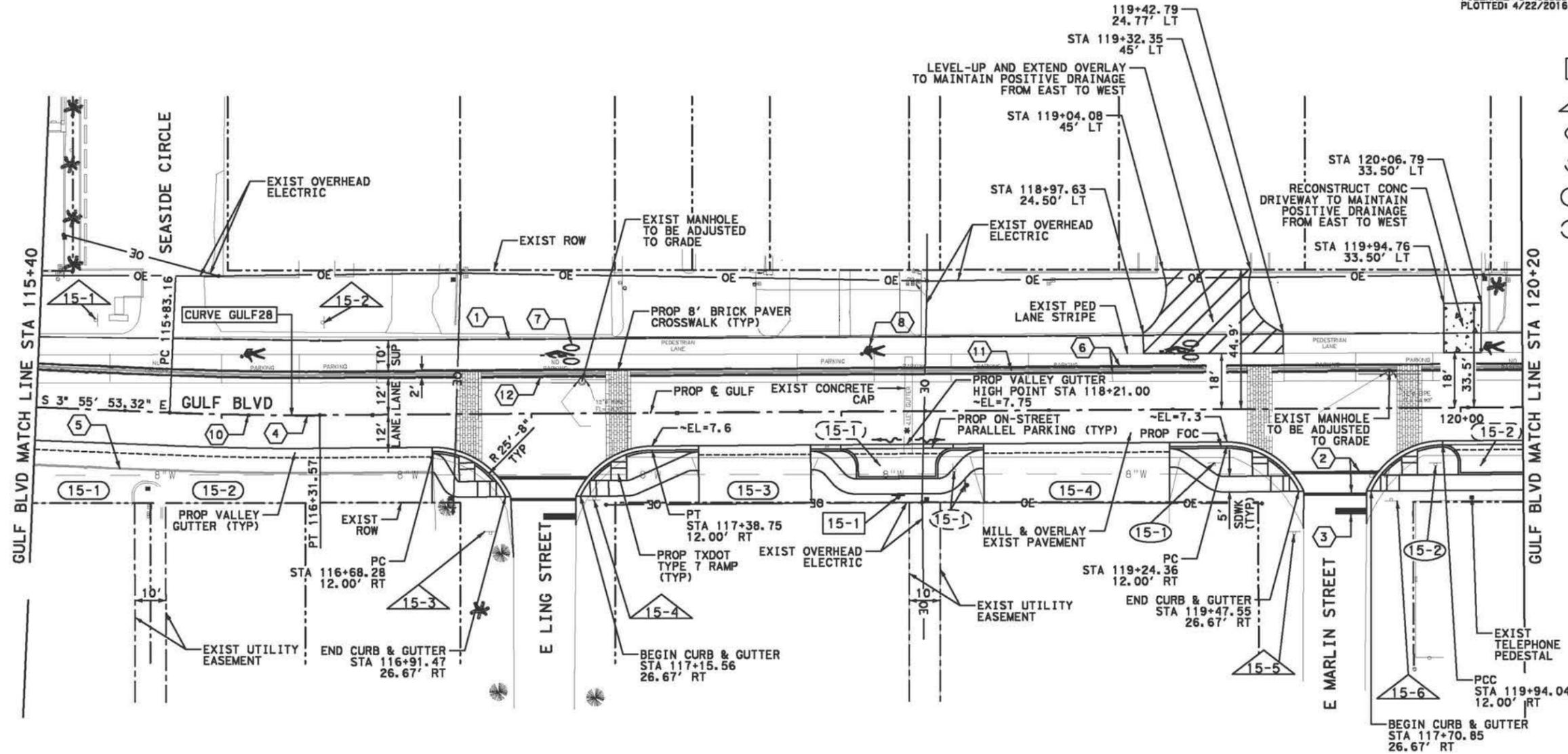
\* VALLEY GUTTER HIGH POINT MATCHES EXISTING PAVEMENT ELEVATION. CONTRACTOR TO SET VALLEY GUTTER GRADES TO MAINTAIN POSITIVE DRAINAGE TO LING ST AND MARLIN ST AS SHOWN. APPROXIMATELY 65 SY OF LEVEL-UP (3" MAX) WILL BE NEEDED BETWEEN THE PROP GUTTER HIGH POINT AND MARLIN ST ALONG WITH BETWEEN THE PROP GUTTER HIGH POINT AND LING ST TO MAINTAIN POSITIVE DRAINAGE.
