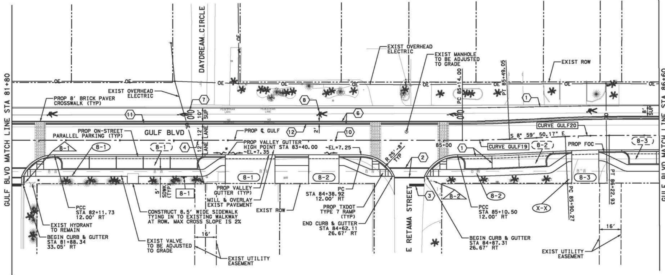
\* VALLEY GUTTER HIGH POINT MATCHES EXISTING PAVEMENT ELEVATION. CONTRACTOR TO FOLLOW EXISTING PAVEMENT SLOPE FROM PROP GUTTER HIGH POINT TO MEZQUITE ST. CONTRACTOR TO ADD APPROXIMATELY 40 SY OF LEVEL-UP (1" MAX) BETWEEN PROP GUTTER HIGH POINT AND RETAMA ST TO MAINTAIN POSITIVE DRAINAGE.
