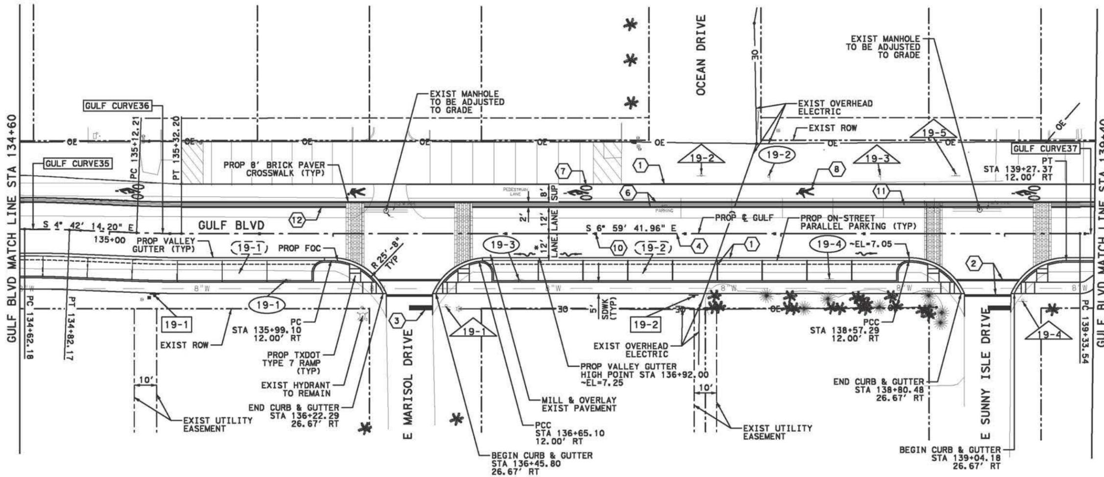
\* VALLEY GUTTER HIGH POINT TO MATCH EXIST PAVEMENT ELEVATION. CONTRACTOR TO FOLLOW EXISTING PAVEMENT SLOPE FROM PROP GUTTER HIGH POINT TO MARISOL DR. CONTRACTOR TO ADD APPROXIMATELY 50 SY OF LEVEL-UP (1" MAX) BETWEEN PROP GUTTER HIGH POINT AND SUNNY ISLE DR TO MAINTAIN POSITIVE DRAINAGE.
