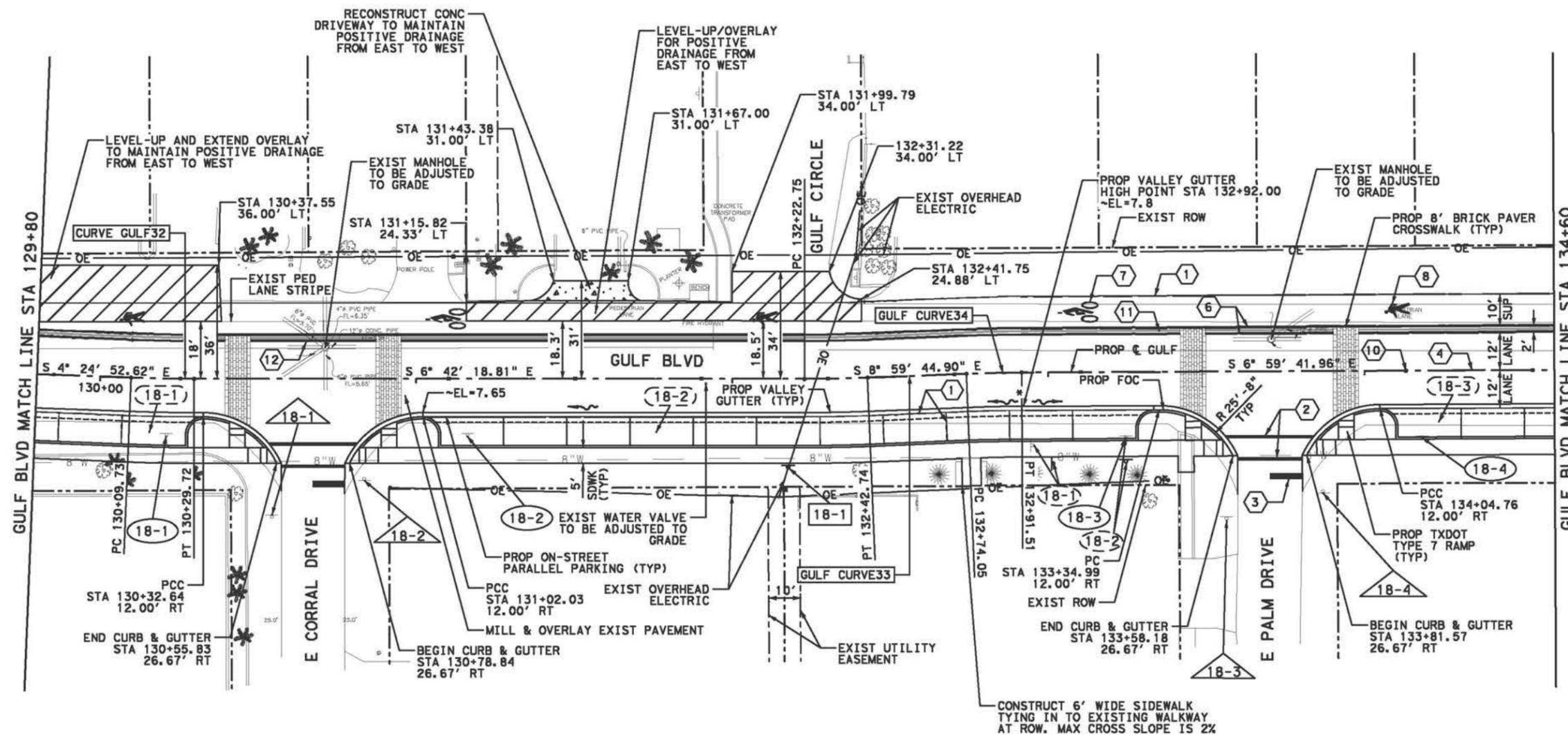
\* VALLEY GUTTER HIGH POINT MATCHES EXISTING PAVEMENT ELEVATION. CONTRACTOR TO FOLLOW EXISTING PAVEMENT SLOPE FROM PROP GUTTER HIGH POINT TO PALM DR. CONTRACTOR TO ADD APPROXIMATELY 114 SY OF LEVEL-UP (2" MAX) BETWEEN PROP GUTTER HIGH POINT AND CORRAL DR TO MAINTAIN POSITIVE DRAINAGE.
