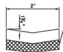
PLACE VALLEY GUTTER ON EXISTING BASE MATERIAL. IF FINAL SURFACE OF BASE MATERIAL IS DISTURBED, CONTRACTOR TO CORRECT SURFACE IN ACCORDANCE WITH SPECIFICATIONS FOR NEW BASE. CONSIDER ANY CORRECTIONS SUBSIDIARY TO PAY ITEM FOR 2' CONCRETE VALLEY GUTTER
