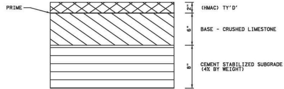
ASPHALT PAVEMENT RECONSTRUCTION SECTION
