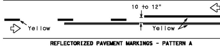
REFLECTORIZED PAVEMENT MARKINGS - PATTERN A
