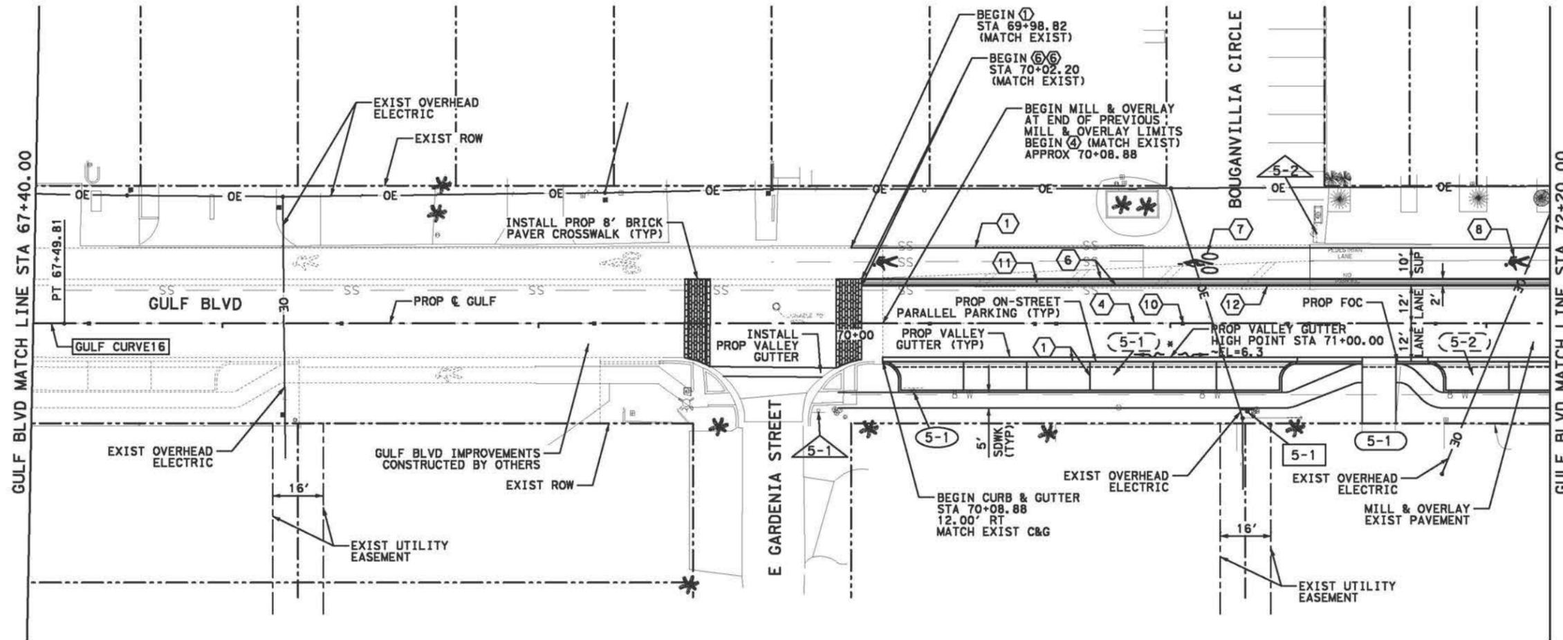
\* PROP VALLEY GUTTER HIGH POINT IS ABOVE EXIST GRADE. CONTRACTOR TO SET VALLEY GUTTER GRADES TO MAINTAIN POSITIVE DRAINAGE TO GARDENIA ST AND OLEANDER ST AS SHOWN. APPROXIMATELY 178 SY OF LEVEL-UP (5" MAX) WILL BE NEEDED BETWEEN PROP GUTTER HIGH POINT AND OLEANDER ST ALONG WITH BETWEEN PROP GUTTER HIGH POINT AND GARDENIA ST.
