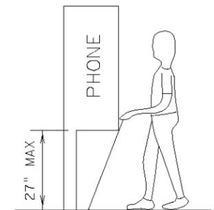
Protruding objects of a height  $\leq 27"$  are detectable by cane and do not require additional treatment.
