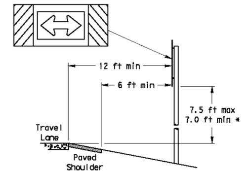
When this sign is needed at the end of a two-lane, two way roadway, the right edge of the sign should be in line with the centerline of the roadway. Place as close to ROW as practical.
