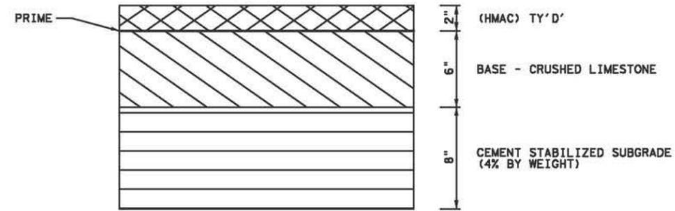
ASPHALT PAVEMENT RECONSTRUCTION SECTION
