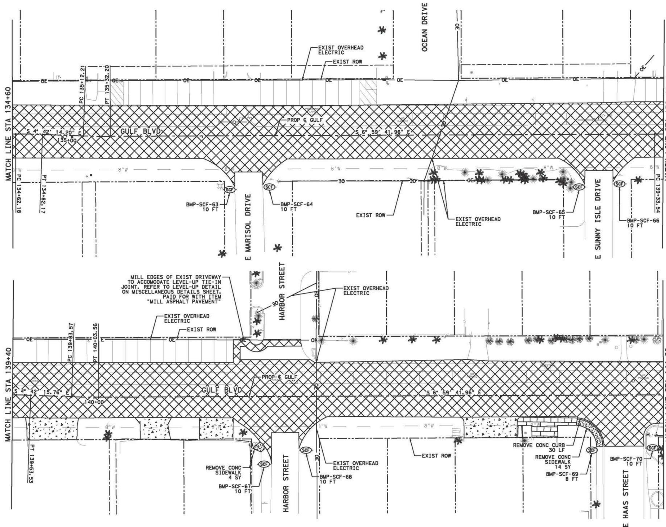
MILL EDGES OF EXIST DRIVEWAY TO ACCOMMODATE LEVEL-UP TIE-IN JOINT. REFER TO LEVEL-UP DETAIL ON MISCELLANEOUS DETAILS SHEET. PAID FOR WITH ITEM "MILL ASPHALT PAVEMENT"
