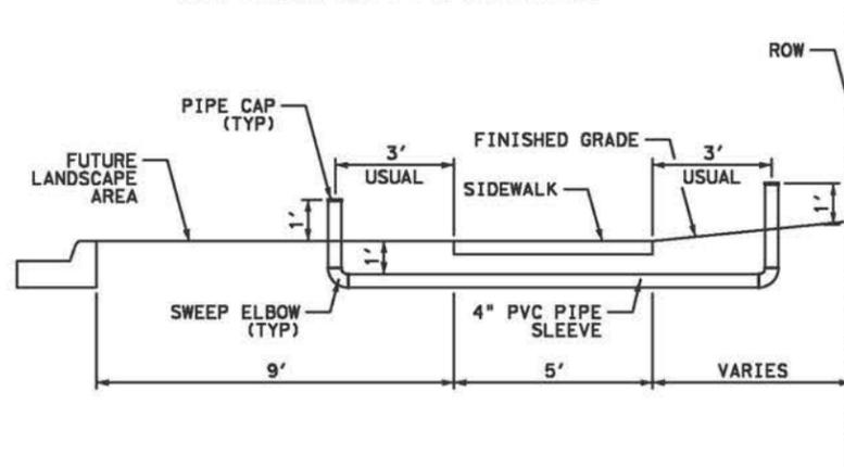
MEDIAN AND IRRIGATION SLEEVE DETAIL
