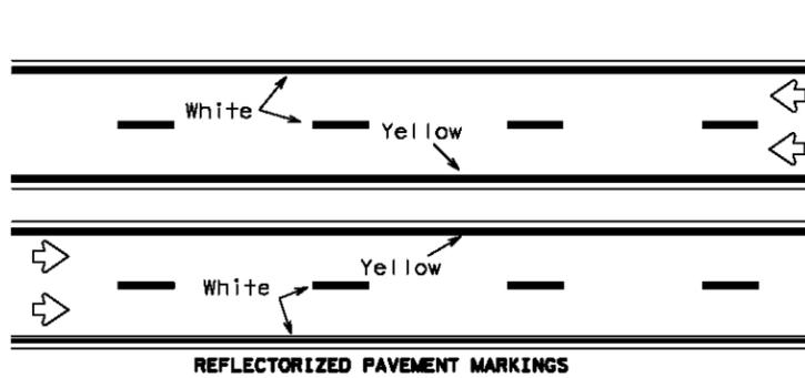
REFLECTORIZED PAVEMENT MARKINGS
