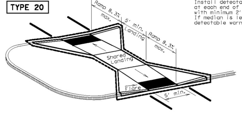
Install detectable warning surface at each end of out-through ramp with minimum 2' smooth surface between. If median is less than 6' wide, eliminate detectable warning surfaces.
