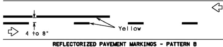
REFLECTORIZED PAVEMENT MARKINGS - PATTERN B
