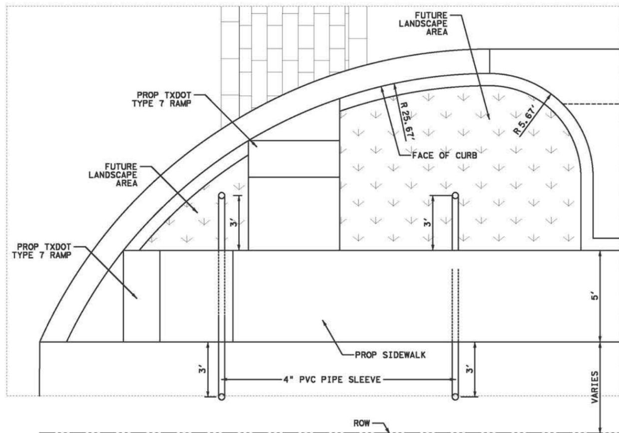
MEDIAN AND IRRIGATION SLEEVE DETAIL
