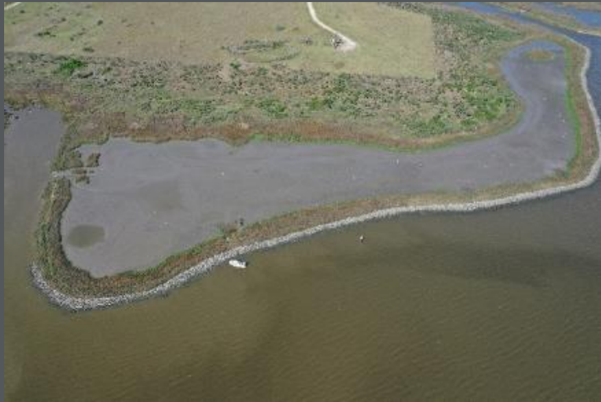
Dickson Bayou – Marsh fill with Riprap protection
