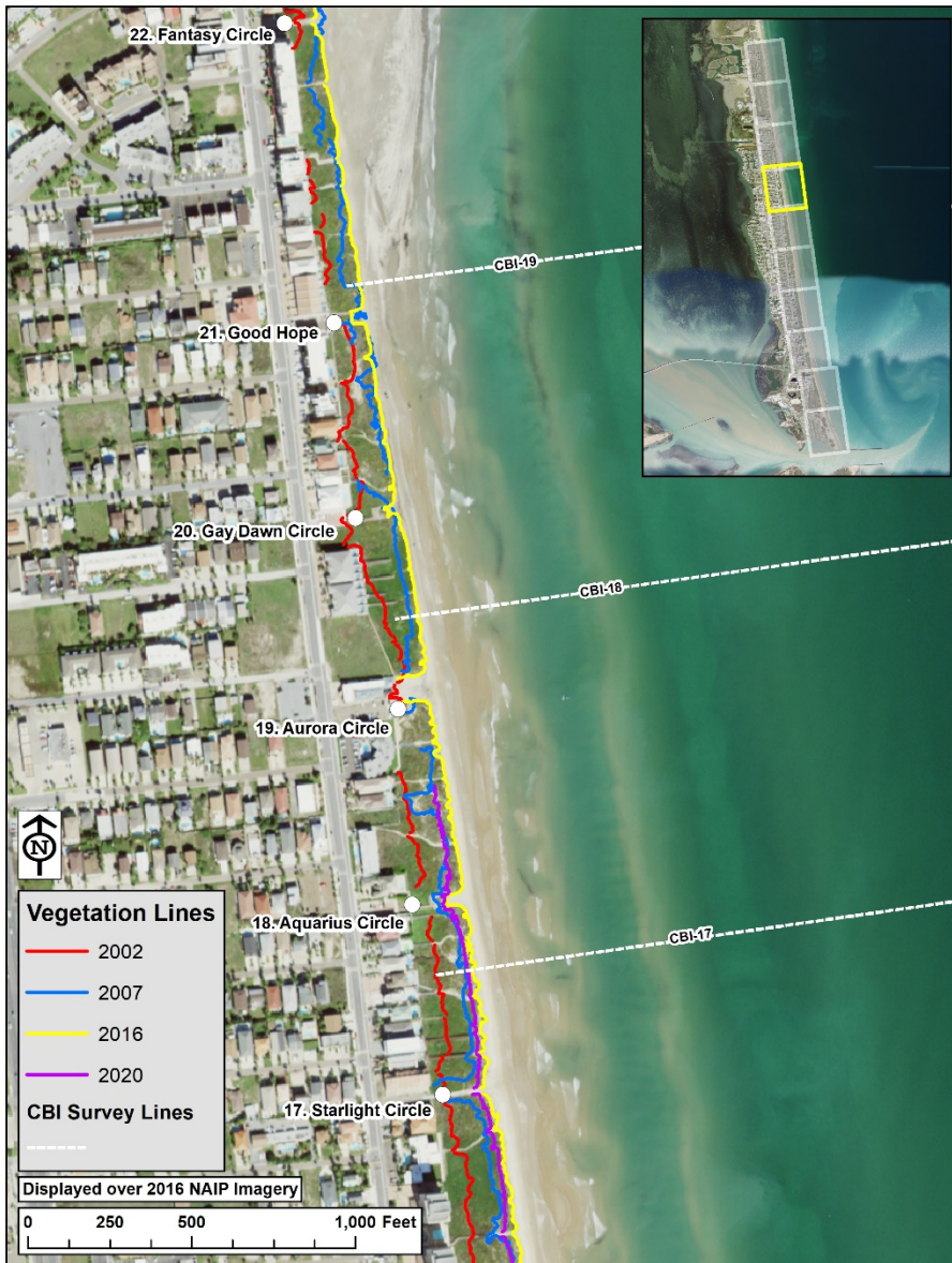
Figure 8-1. A north-central section map showing vegetation lines from 2002–2020. Note the 2020 line ends between CBI-17 and CBI-18. This map is also provided at full scale in Appendix D. The dots and numbered place names are the names of beach access locations at SPI.
