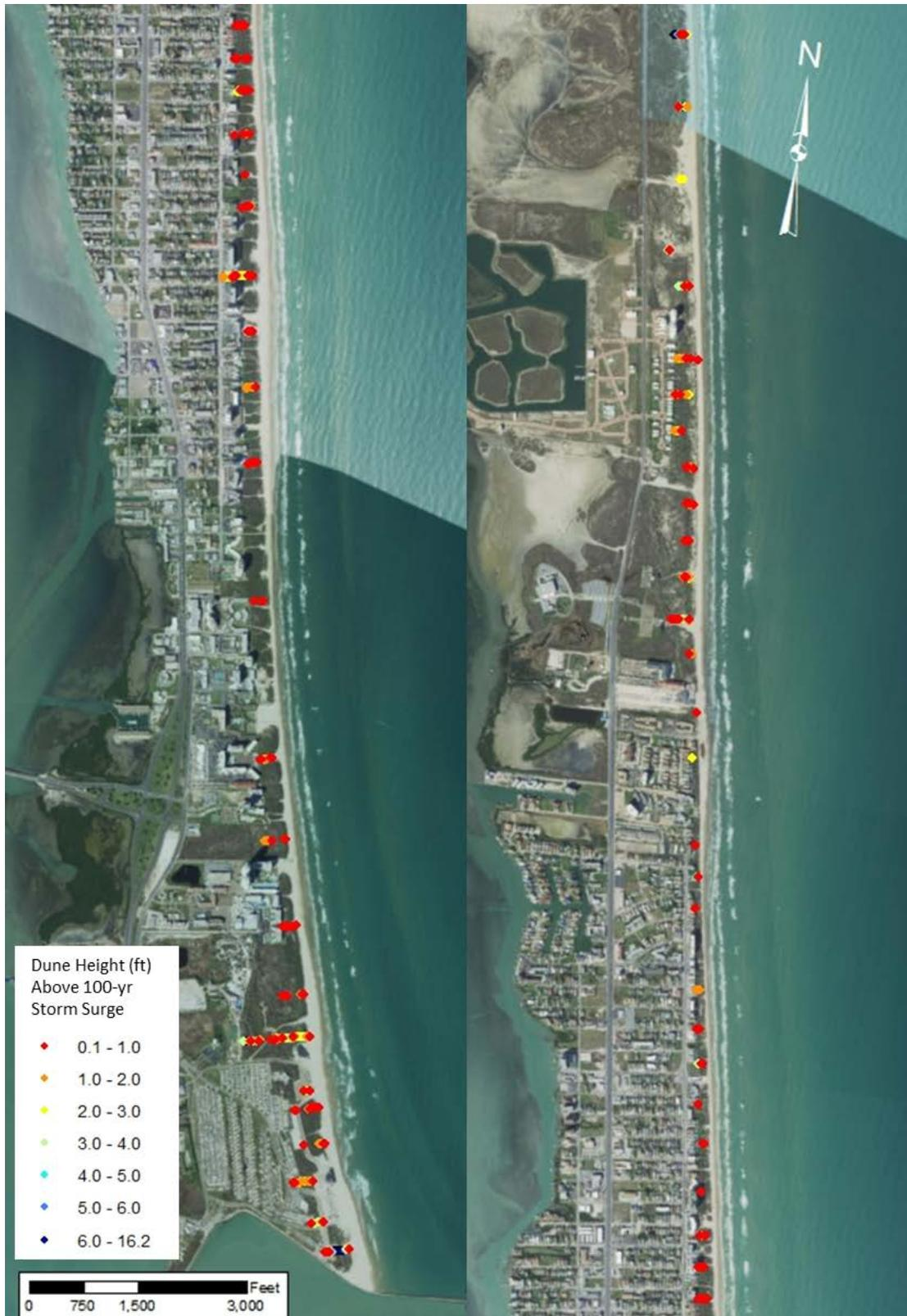
**Figure 4-6. Existing Dune Height Exceeding 100 year Storm Surge Elevation of +9.3 ft NAVD**
